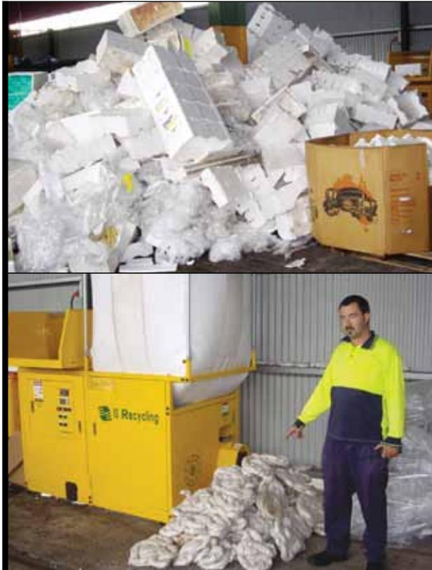
Foam boxes are volume reduced by 90 times to recyclable ingots.
